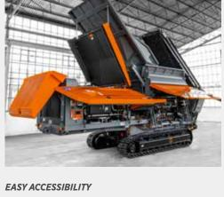
The lightweight GRP doors open upwards so that you always have easy access to all sides. With the Inventhor 6.2, you also have the option of folding up the GRP roof using the feed hopper to further improve accessibility.
